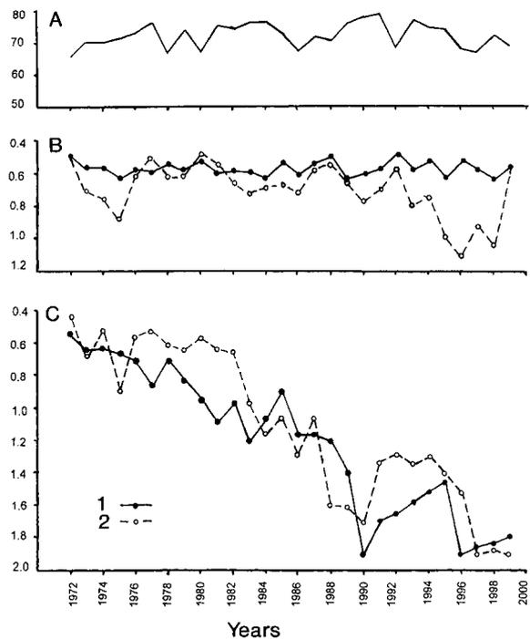
Figure 4 Changes in (A) index of thawing overtime ( $^{\circ}\text{C}\cdot\text{day}^{\frac{1}{2}}$ ), and (B) the active layer thickness (m) in natural (undisturbed) sites and (C) in disturbed sites, at the Nadym geocryological station, 1972–1999. 1—flat-topped peat bog; and 2—bog with small peat mounds.
