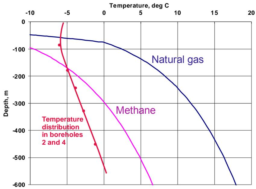
Figure 2. Equilibrium curves for natural gas and pure methane. Temperature distribution within South Tambej gas field is shown according to Kondakov et al., 2011.
