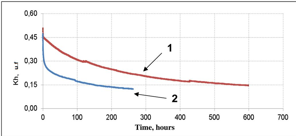
Figure 5. Dissociation kinetics of methane's hydrate in examples of the frozen artificially hydrate-saturated sediments at pressure decrease in sand to 1,3 MPa (1), sandy loams to 0,6 MPa (2) at a temperature of -5,2 °C.
