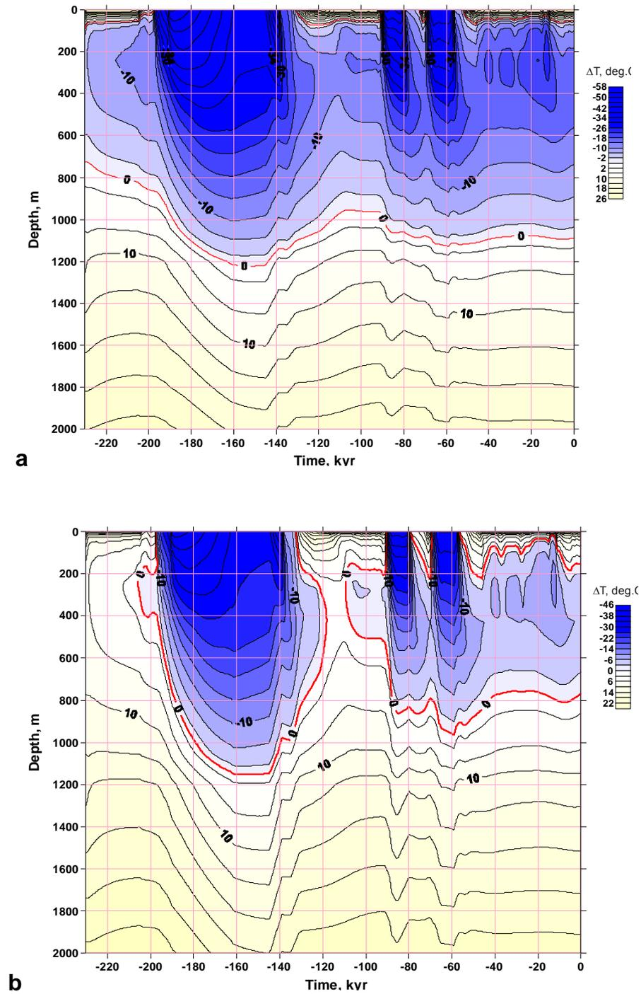
Figure 4. The evolution of gas hydrate stable zone: a - for natural gas composition, b - for pure methane.
